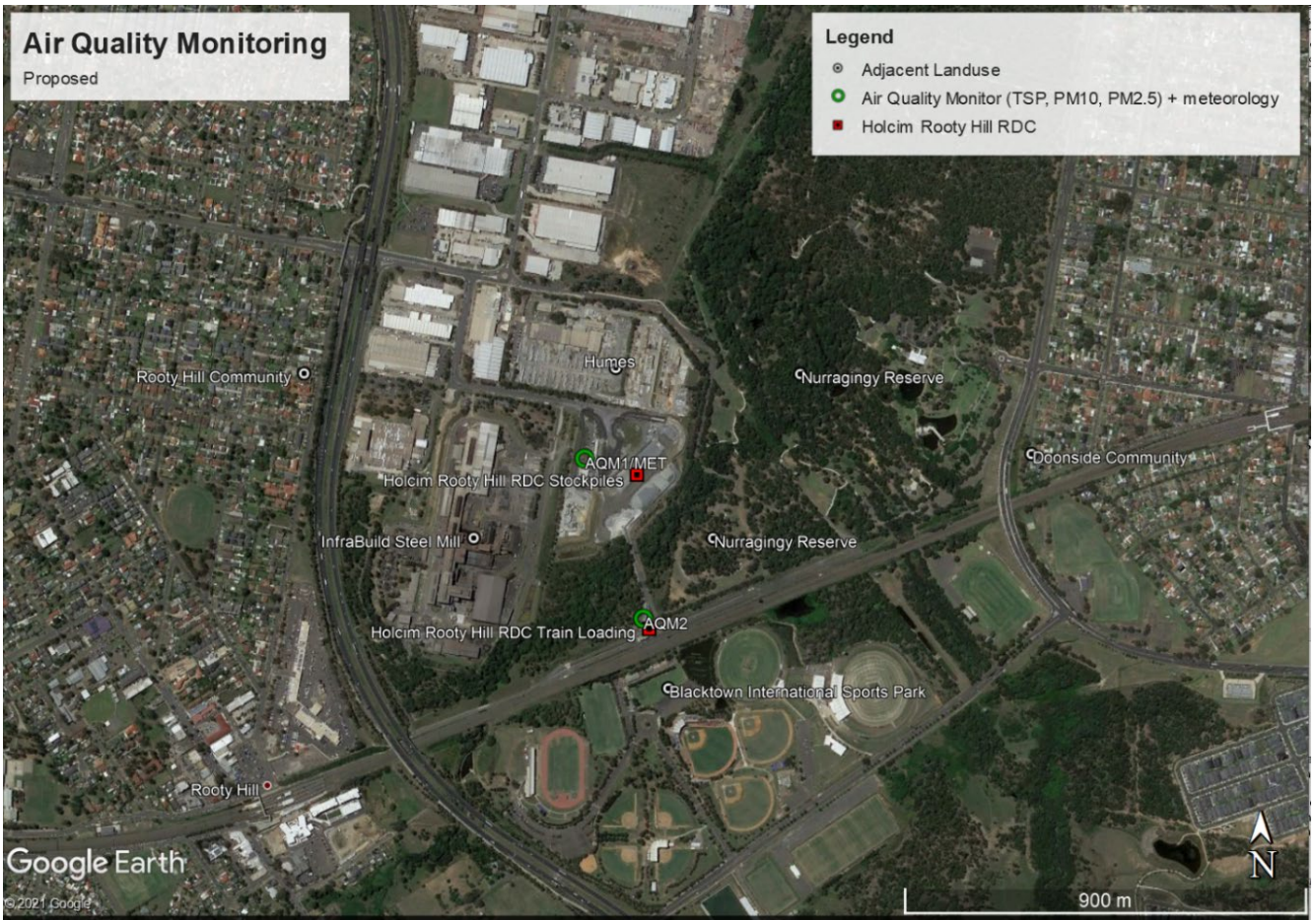
Figure 4-1: Proposed air quality monitoring program at Holcim RHDC with surrounding land uses (Google Earth, 2021)
